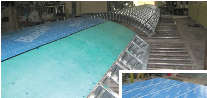
Curved & Straight Panels assembled with Densglass sheathing and Blueskin SA.
