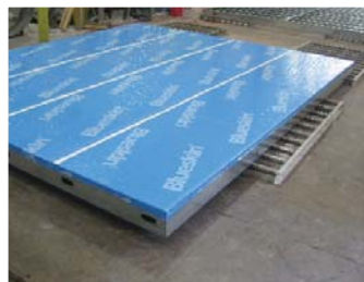
Curved & Straight Panels assembled with Densglass sheathing and Blueskin SA.
